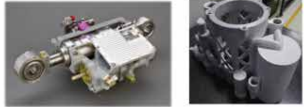
Hydraulic Flight Control Actuator & Additive Manufactured Manifold
