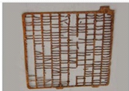
Corroded positive grid from a conventional lead acid battery
